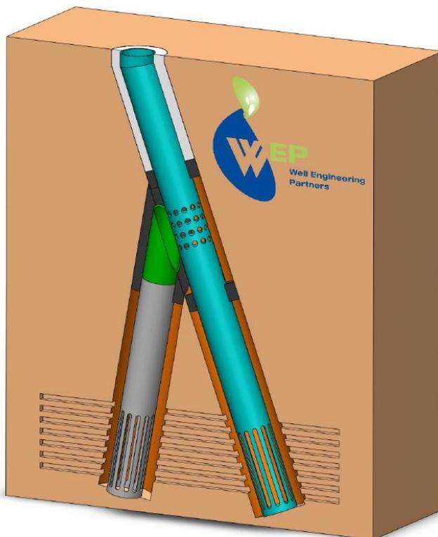
Figure 4: Schematic multilateral well completion as proposed in the RESULT project
