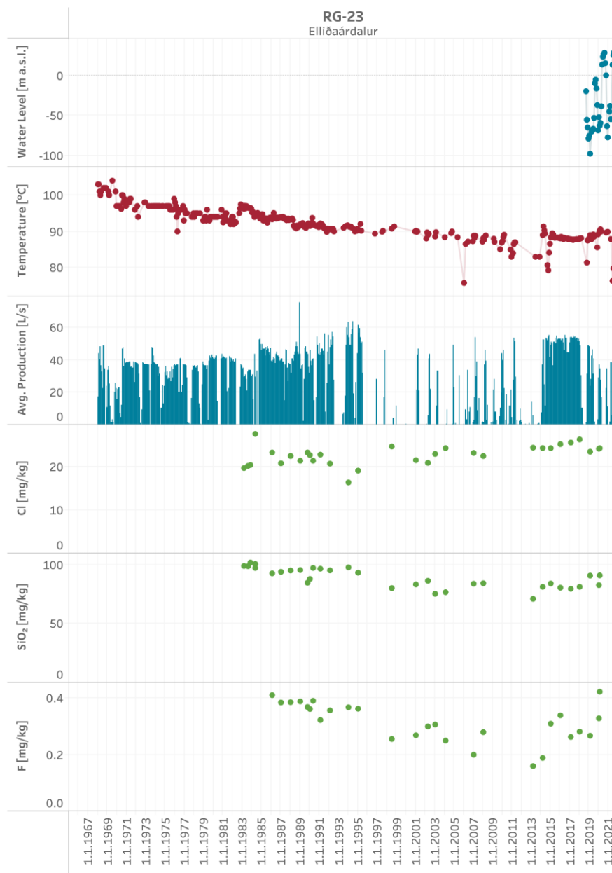
Figure 6. Water level data, temperature of produced fluid, average production, and concentration of Cl, SiO 2 and F in produced fluid from RG-23.
