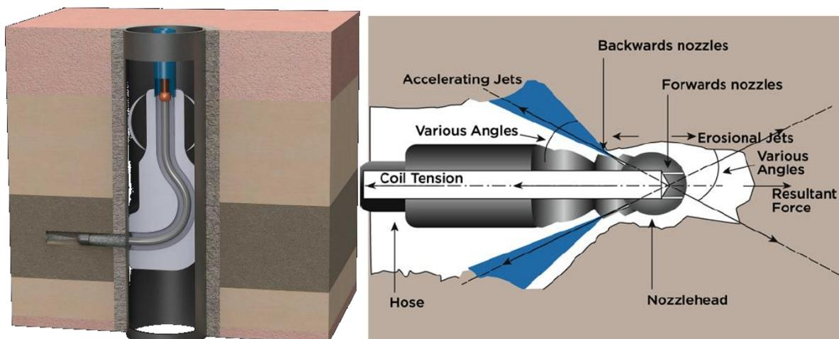
**Figure 15.** *Left: A deflector shoe is placed in the wellbore and coil tubing with attached nozzle feed led through it and directed towards the wall of the borehole (Reinsch & Blöcher, 2017). Right: setup of a nozzle head used in radial jetting (Peters et al., 2015).*
