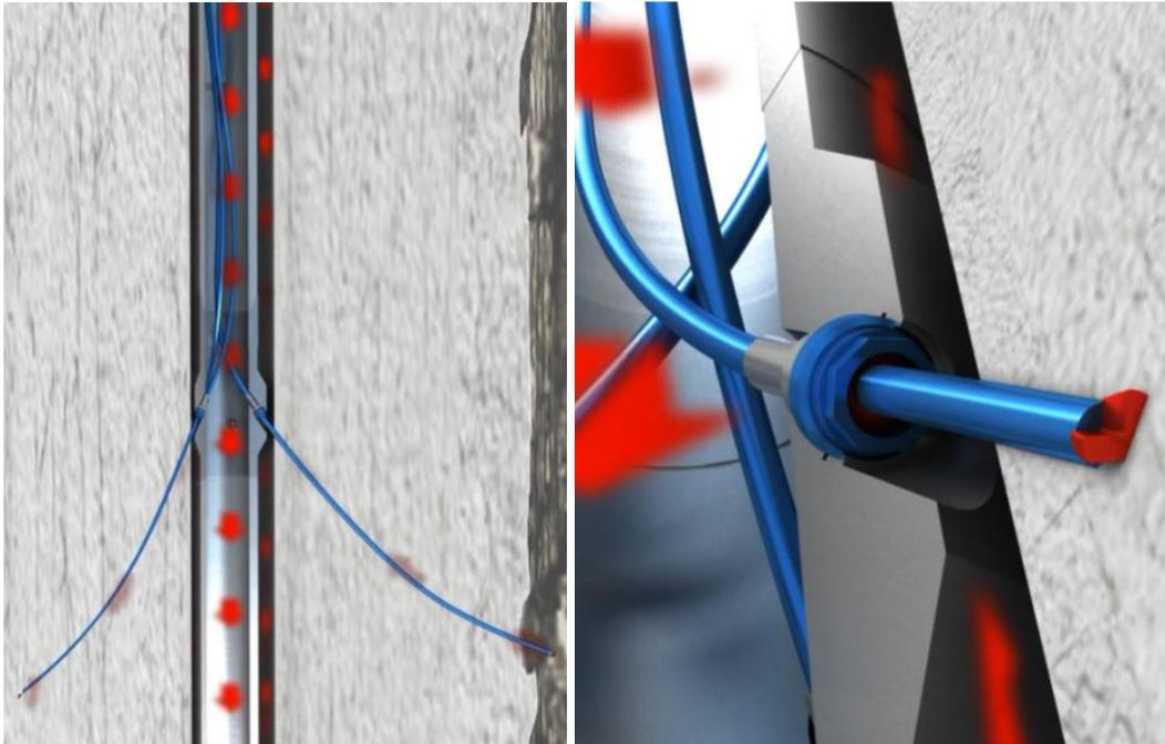
**Figure 16.** Fishbone drilling (<https://www.fishbones.as/drilling>).
