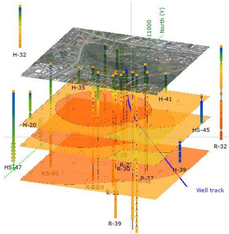
**Figure 19.** *Speculations on potential well track to the northeast using directional drilling.*
