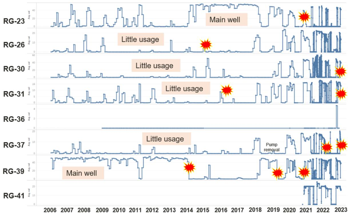
**Figure 13.** Pump failures (red symbols) due to corrosion or scaling in the Elliðaárdalur production wells between 2006 and 2023 shown on a production graph (L/s) for each well.
