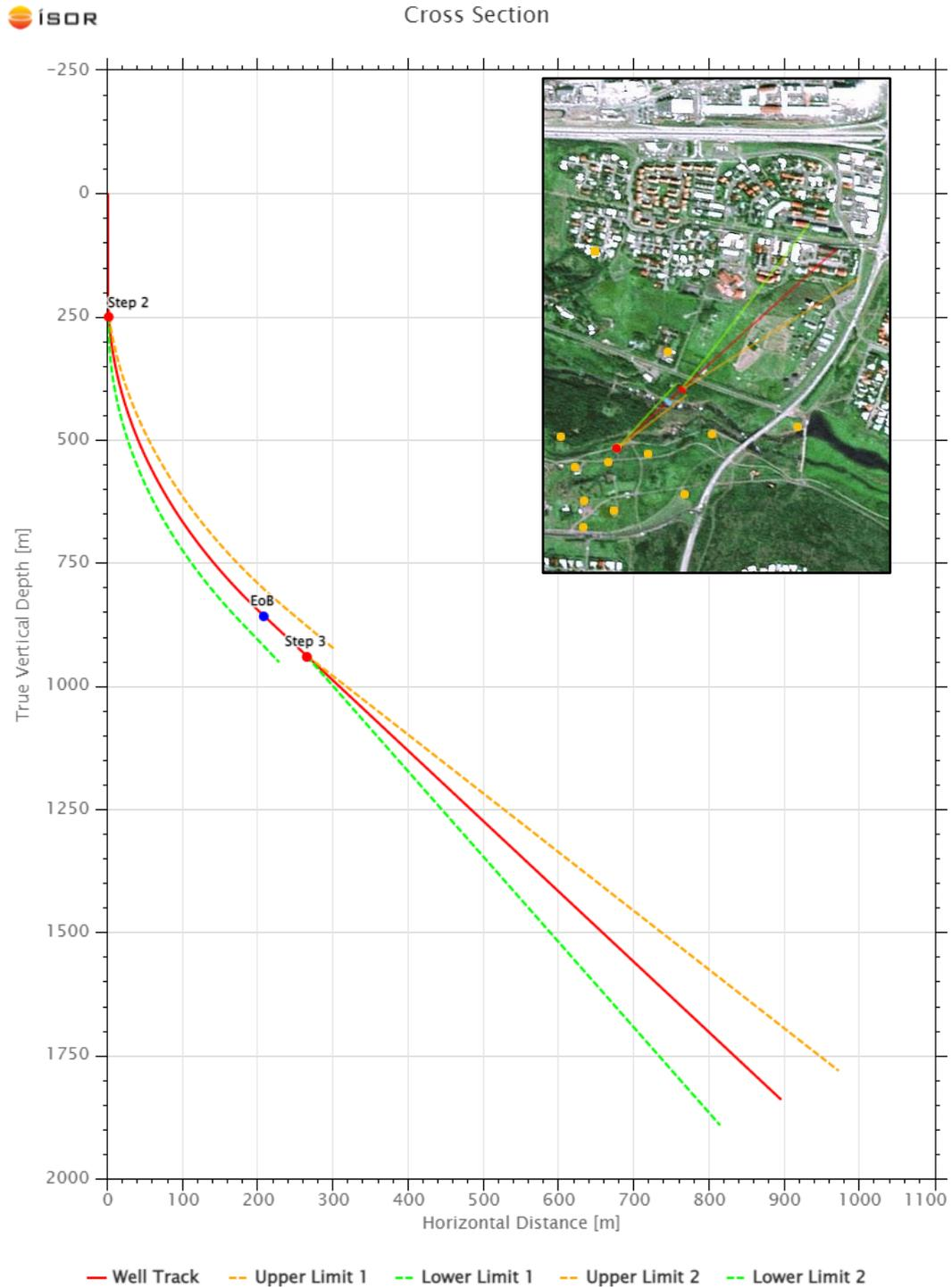
**Figure 18.** Speculations on directional drilling that could provide extended reach below Elliðaár river and residential area (Ártúnsholt) to the northeast where temperature model shows increased temperature.
