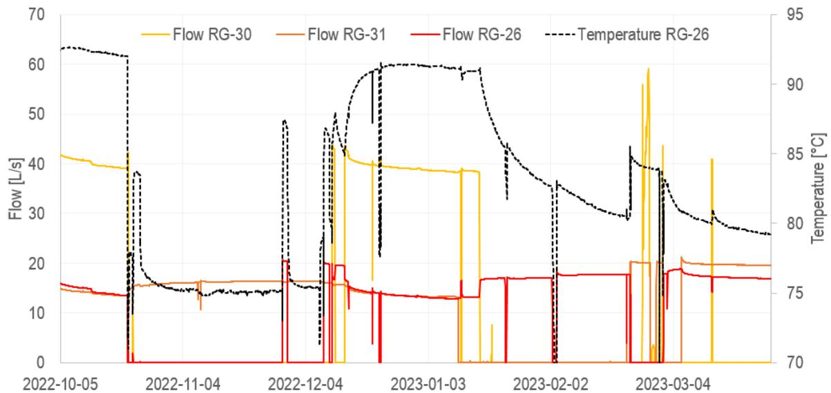
**Figure 12.** Changes in production temperature for well R-26 corresponding to changes in flow from wells R-30, R-31 and R-26.
