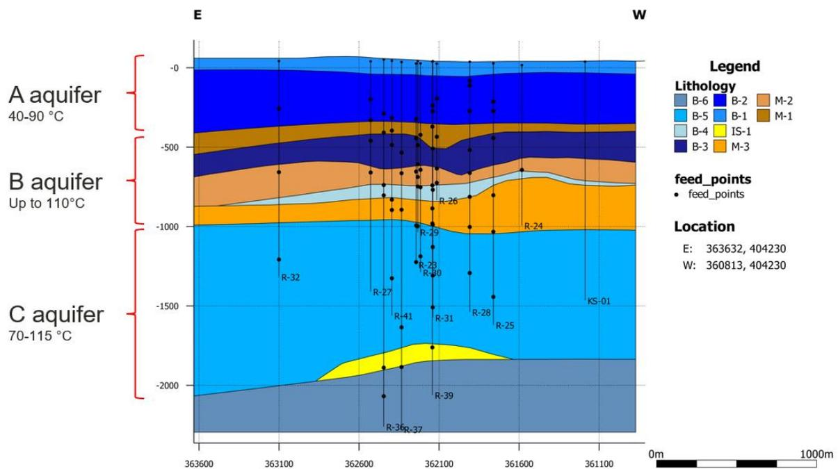
**Figure 2.** An E-W cross section through a geological model of the Elliðaárdalur field. B-formations are basalt lava flows and M-formations are hyaloclastite formations. Feed points identified are shown for each well. The division into aquifers and the corresponding temperatures are from Tómasson (1988).
