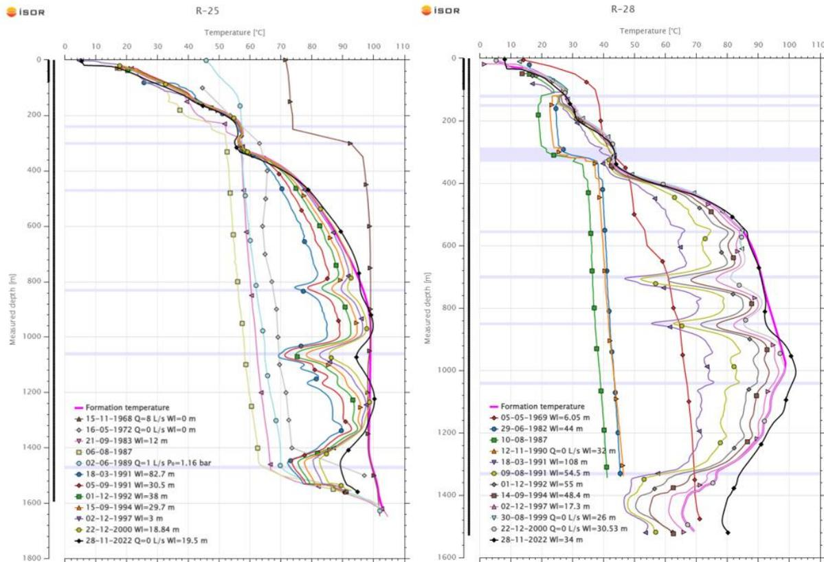
**Figure 8.** Downhole temperature logs and estimated formation temperature for wells R-25 (left) and R-28 (right). The estimated feed zones in the wells are shown as blue shading, and the well casings are indicated as black vertical lines on the left. Both wells were sealed with monitoring pipes in 1991.
