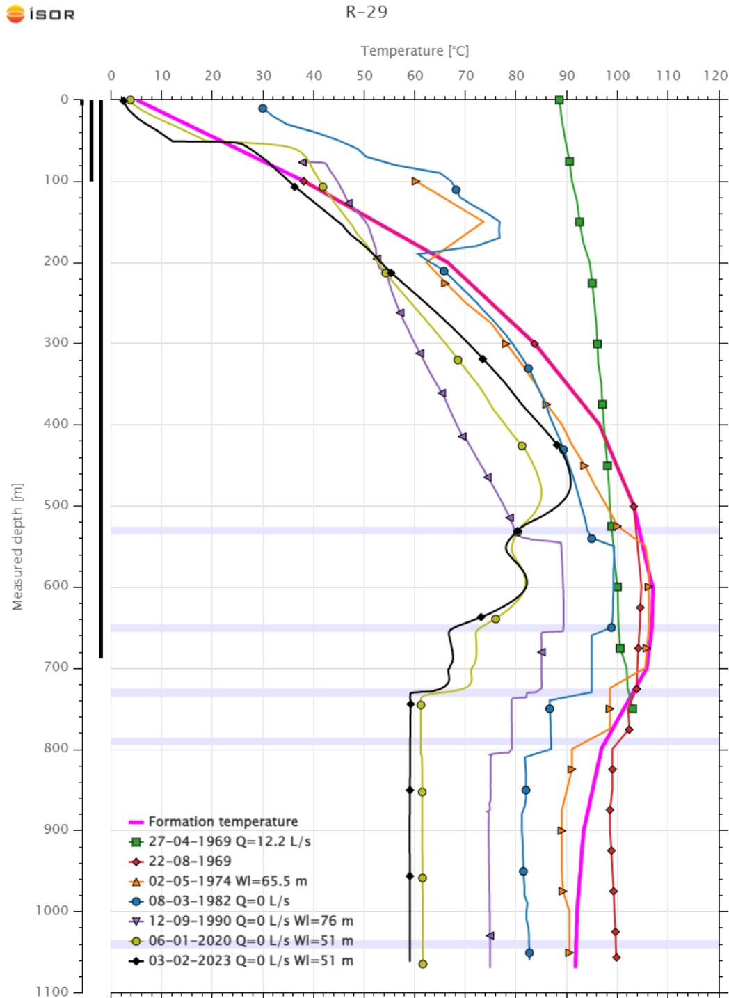
**Figure 9.** Downhole temperature logs and estimated formation temperature for well R-29. The estimated feed zones in the wells are shown as blue shadings, and the well casings are indicated as black vertical lines on the left.
