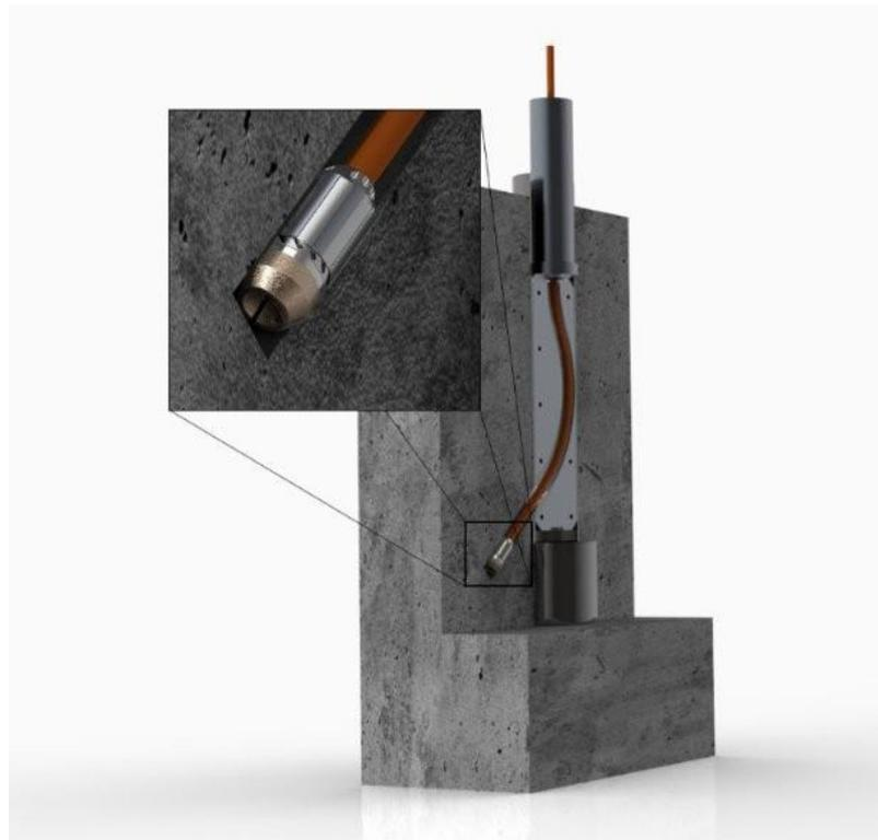
**Figure 17.** Micro-turbine tool. Deflection shoe directing the drilling tool outwards at a 45° angle (Fero, 2022).
