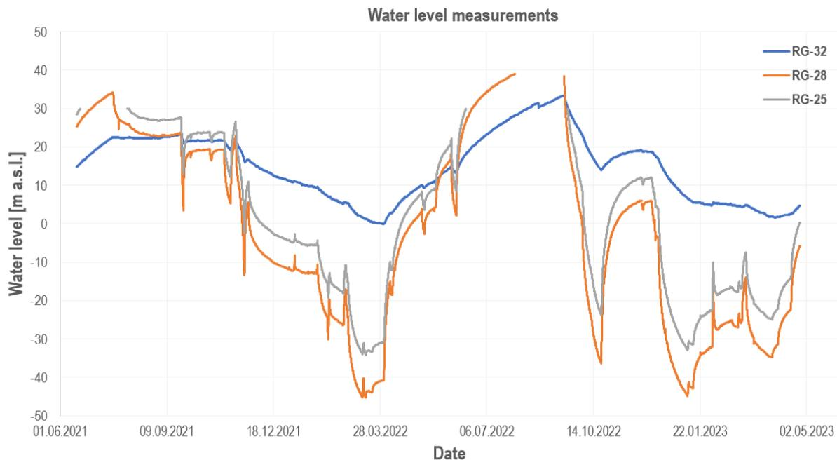
**Figure 14.** Water level measurements in well R-32 located 1.5 km to the northeast of the production zone and wells R-28 and R-25 located at the southwestern edge of the production zone.
